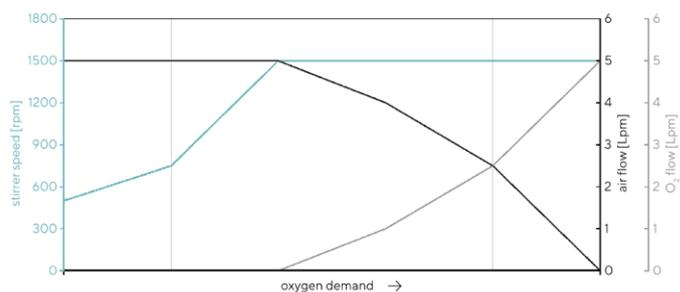
**Figure 1:** Schematic pO<sub>2</sub> cascade of both cultivations. Starting with a constant air gas flow of 5 lpm, pO<sub>2</sub> was controlled by increasing tip speed to 1500 rpm and supplementing oxygen.
