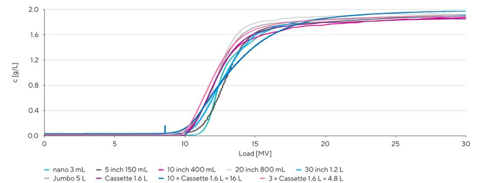
Figure 6: BSA breakthrough curves of void volume optimized capsules and single, 3 + 1.6 L cassette and 10 x 1.6 L cassette, 8 mm bed height versions.
