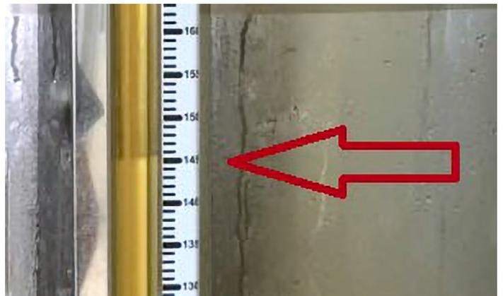
Figure 3: Separation between filtered and unfiltered beer
