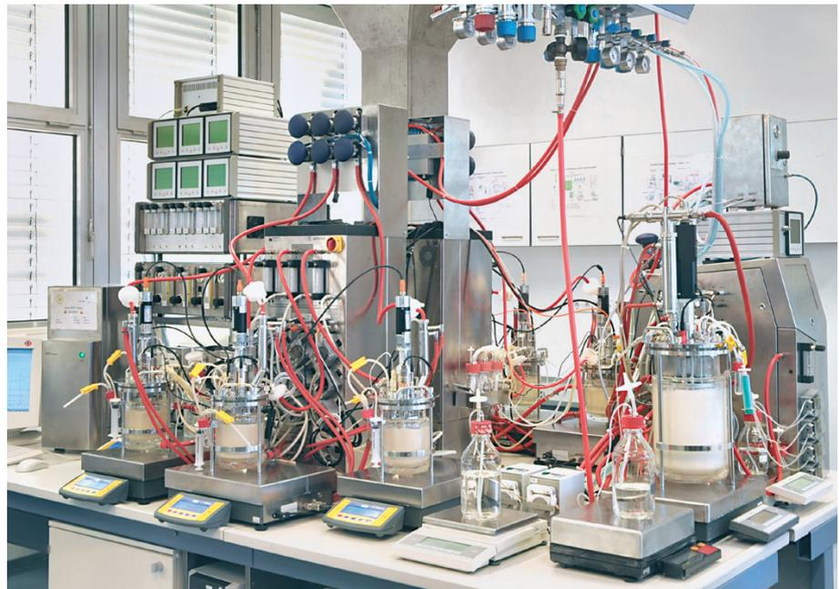
Fig. 1: Multi-bioreactor DoE-plant with BIOSTAT® Bplus and Qplus
