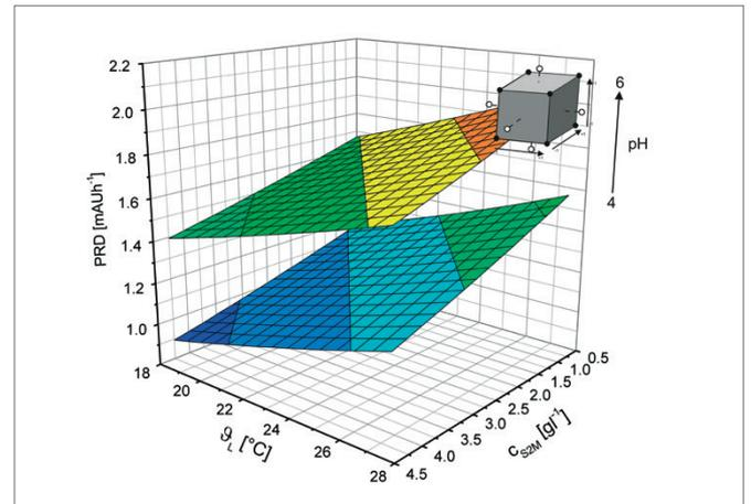
Fig. 4: Response surface plot of DoE-Screening of productivity (PRD) as a function of methanol concentration ( $c_{S2M}$ ) and cultivation temperature ( $\vartheta_L$ )
