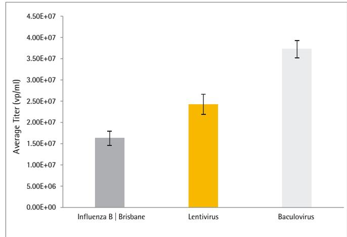
Figure 3: Optimal dilution within the linear range of the instrument was chosen to determine sample counts in replicates of five. Measured coefficients of variance (CVs) are 10.3% (Influenza B), 10.1% (Lentivirus) and 5.7% (Baculovirus).
