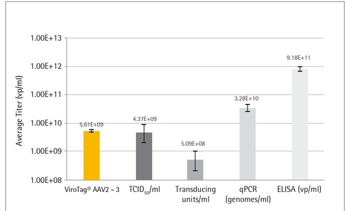
Figure 6: ViroTag AAV 2/3 was used with other quantification methods to quantify AAV 2 virus standard (ATCC). CV for Virus Counter platform measurement 2.79 %. CVs measured for other methods from left to right 374 % c.v., 192 % c.v., 109 % c.v., 29.0 % c.v. Data from Lock *et al.*
