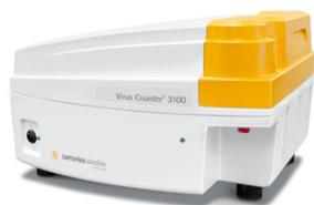
The Virus Counter<sup>®</sup> instrument detects viral particles in a fluid stream.
