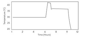
Process required precision temperature control and high stir speed. Fast temperature rise in the bag followed by fast temperature drop were required to achieve optimal conditions for induction of product synthesis in the fermentation broth.
