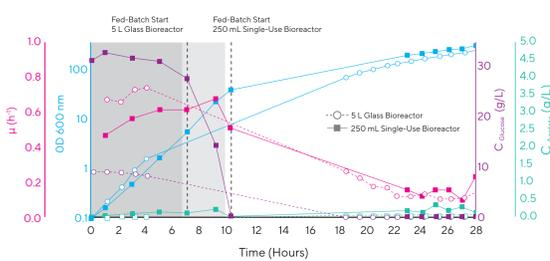
Note. Ambr® 250 Modular run (squares) compared with a Univessel® Glass 5 L reactor (circles); optical density at 600 nm (blue), growth rate (dark pink), acetate (teal), and glucose concentration (purple). Dashed line indicates feed
