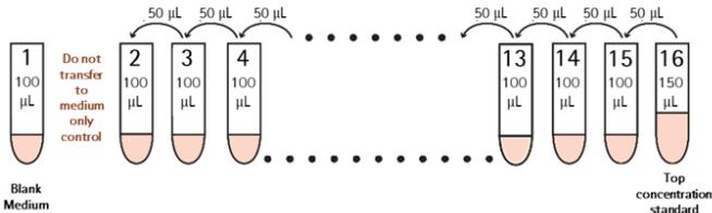
**Figure 7.** Serial dilution of Cytokine Standards. For both 96- and 384-well formats, Cytokine Standards are to be serially diluted 1:3 by adding 50  $\mu$ L from the top concentration standard into 100  $\mu$ L of culture medium serially. A blank medium tube should be included as a control.
