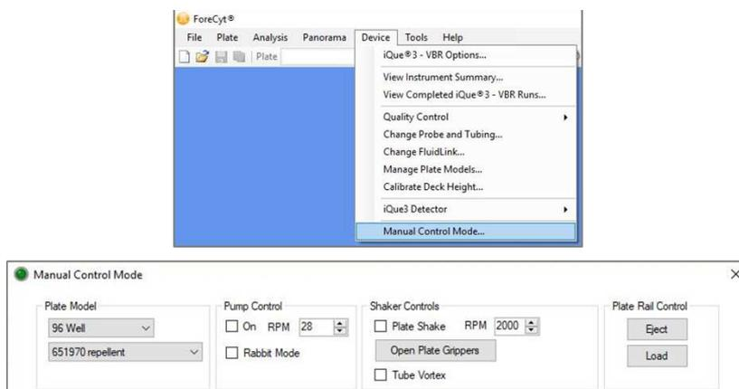
**Figure 12.** Steps for using the shaker on iQue®3 (VBR) or iQue® Screener PLUS (VBR). Set the shaker speed to either 2000 RPM or 3000 RPM depending on the assay requirements. It is important to note that shaking at 3000 RPM is reserved only for the step post-aspiration. Shaking the plate at 3000 RPM with liquid in the wells will result in cross-contamination.
