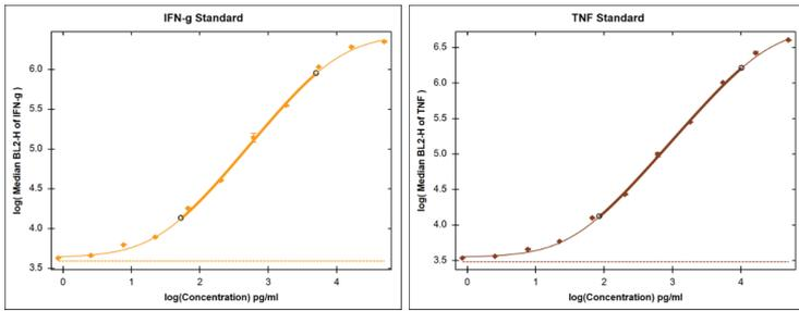
**Figure 6.** Representative standard curves (IFN $\gamma$  and TNF) with 1:3 serial dilutions. The bold lines indicate the linear range in each graph, with the detection range wider than the linear range. The linear ranges for IFN $\gamma$  and TNF are 55–5,000 pg/mL, and 85–10,000 pg/mL, respectively. The dashed line represents the fluorescent background when the standard concentration is zero.
