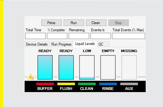
Automated data analysis and tracking of QC functionalities allows identification of potential instrument performance issues before running precious samples.
