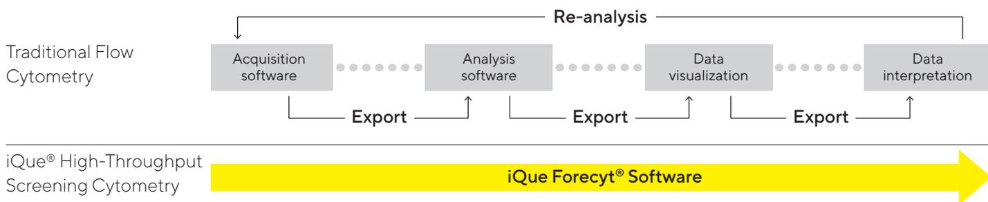
Traditional flow cytometry data analysis workflows versus one unified workflow using iQue Forecyt® Software. Traditionally scientists have been required to export and import data between several software packages in order to go from acquisition to analysis to data visualization and even to statistical packages for interpretation of their data. iQue Forecyt® Software provides all of this functionality in a single easy-to-follow workflow to get to actionable answers in record time.
