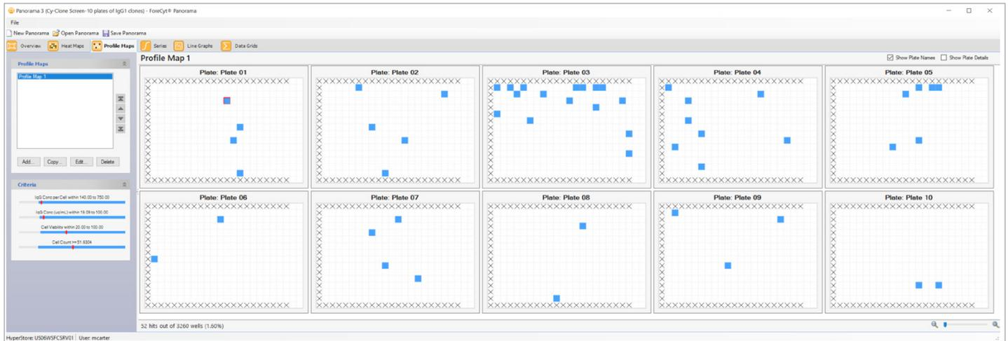
Panorama view: Easily visualize “hits” across multiple plates according to different metrics. In this example 10 plates were analyzed simultaneously using the Cyclone Plus kit which correlates IgG titer-per-cell with cell health information and cell growth readouts. The wells which meet the user-identified selection criteria are highlighted instantly for each plate.
